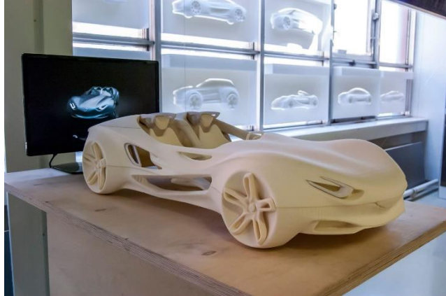
Figure 2 - SLA 3D Printing car prototype. Source: ZONGHENG3D on https://www.zongheng3d.com/from-concept-to-reality-building-functional-prototypes-with-sla-3d-printing/
